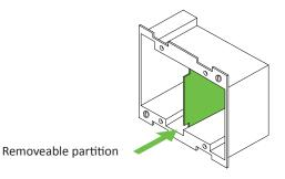
Install gang boxes that include vertical partitions (available at local electrical distributor) unless Class 2 circuit conductors are installed in accordance with 725.41 Class 1 Circuits.
