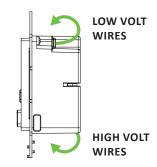
For extra shallow wall boxes it's acceptable to use the dimmer housing as a barrier. Tuck wires on top and bottom sides of dimmer housing.
